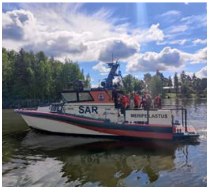
The Finnish-built "Tervasaari" has a length of 13.5 metres, a width of 4.5 metres, a weight of 15 tonnes and a speed of 30 knots.
