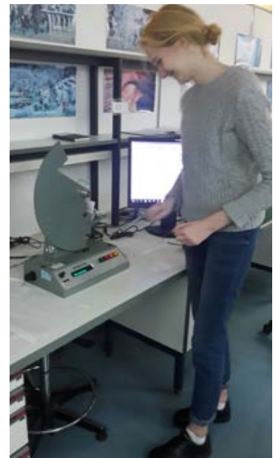
Aela Norris performing tear testing
