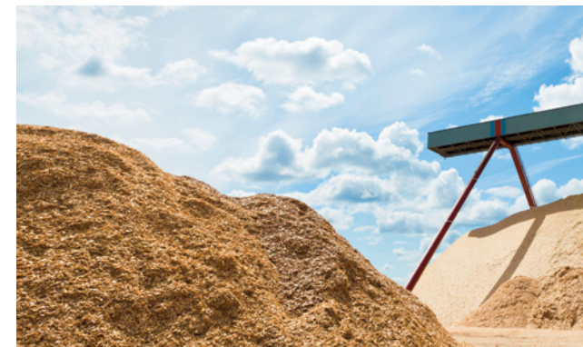
Pine, spruce, birch and eucalyptus are the raw materials used for the production of sulphate pulp. The debarked wood is chipped and screened before the pulp cooking process. The picture shows the pine, spruce and birch chip stores at the UPM Kymi pulp mill in Finland.
