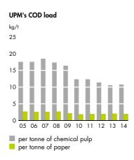
The COD load has decreased by 26% per tonne of paper, and by 39% per tonne of chemical pulp, over the last ten
