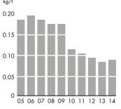
AOX indicates the amount of halogens bound to the organic compounds present in the effluent. Over the last ten years, the AOX load per tonne of bleached chemical pulp has decreased by 53%.
