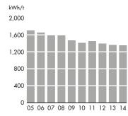
The electricity consumption per tonne of paper has decreased by 20% over the last ten years due to continuous improvements in energy efficiency.
