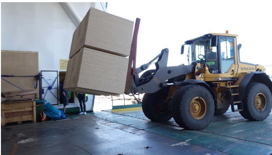
Picture 3. Forks suitable for single pack handling
