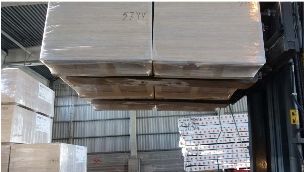
Picture 2. Forks suitable for multipackage handling
