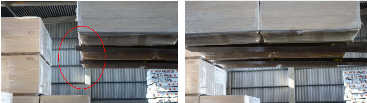
Picture 1. Forks protruding pallets causing risk to damage pallets behind.
